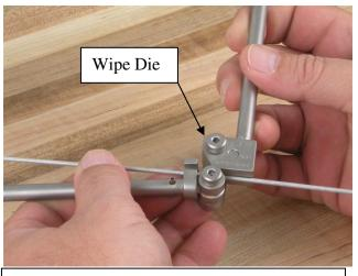
Figure 2: While holding up the back stop with your left hand, close the wipe die with your right hand until it sits tangent to the coax.
