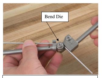
Figure 3: Rotate the wipe die handle CW about the bend die until the desired bend angle is achieved.
