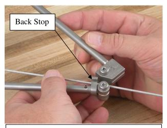
Figure 1: Install coax in bend die groove and then rotate up the back stop as shown with your left ring finger or middle finger as shown.
