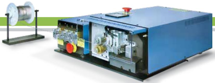
Winton's bench-top cut-off machine is an automatic feed and cut, designed specifically for cutting semi-rigid coax cable.
