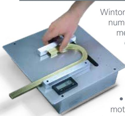
Winton's patented AM40 is a digital protractor designed to measure the bend angle of numerous bend configurations. Its measuring range is from 0 to 360 degrees in increments of 0.1 degrees, and uses a high-resolution encoder to ensure the repeatability of the bend angle measurement. The digital readout, displayed in large numerals, updates continuously to show the real-time bend angle.
